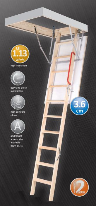
Maximum loading150 kgLadder width38 cmTread width8 cmTread length34 cmDistance between treads25 cmHatch thickness3.6 cmBox height14 cmHeat transfer coefficient\*U=1.13W/m²K
