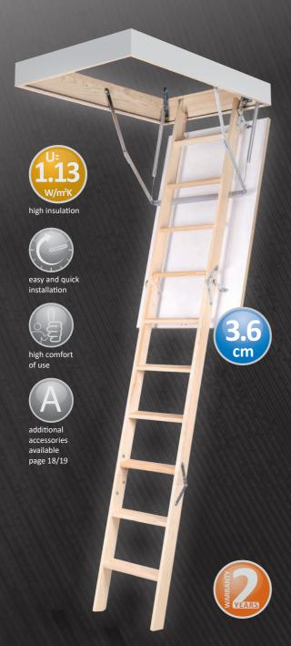
150 kg Maximum loading Ladder width 38 cm Tread width 8 cm Tread length 34 cm Distance between treads 25 cm Hatch thickness 3.6 cm Box height 14 cm Heat transfer coefficient\* U=1.13W/m<sup>2</sup>K
