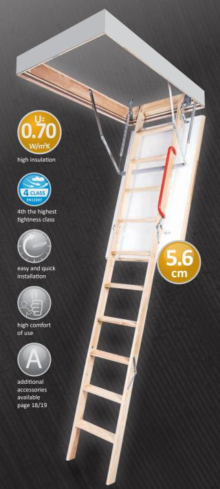
150 kg Maximum loading Ladder width 38 cm Tread width 8 cm Tread length 34 cm Distance between treads Hatch thickness 25 cm 5.6 cm Box height 14 cm U=0.70 W/m<sup>2</sup>K Heat transfer coefficient\* Tightness class\*\* 4th according to EN12207
