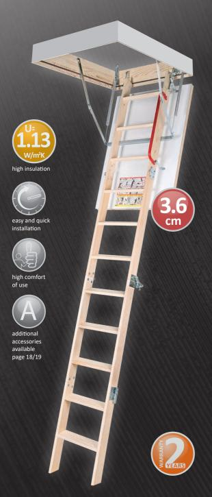
150 kg Maximum loading Ladder width 38 cm Tread width 8 cm Tread length 34 cm Distance between treads 25 cm Hatch thickness 3.6 cm Box height 14 cm Heat transfer coefficient\* U=1.13 W/m<sup>2</sup>K
